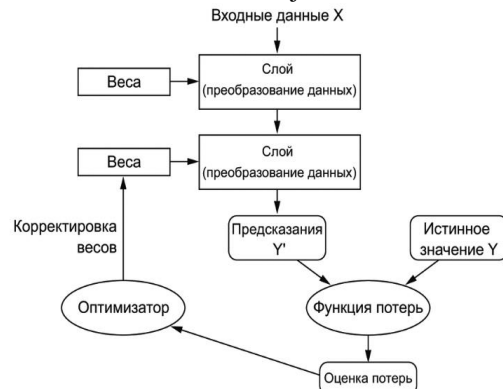
Fig. 2 The loss function evaluates the quality of the results produced by the neural network
