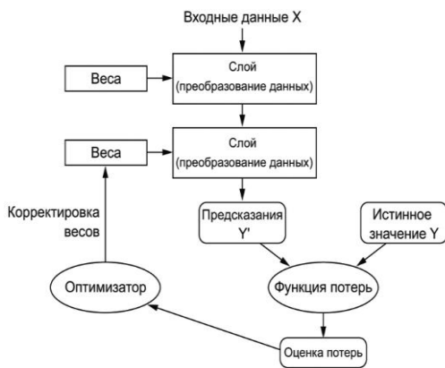
Fig.4 Loss estimates are used as feedback for weight adjustments
